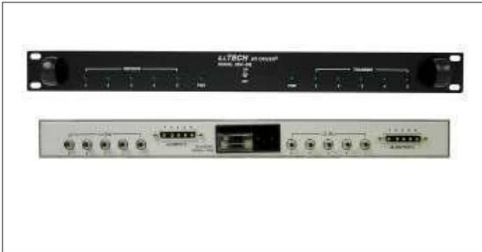
The S.I.Tech Model 2861 is designed for high speed RS-422 and TTL data communication using fiber. This system uses special 5 coax connectors for interfacing to high speed network. Model 2861 provides 5 independent channels for data, clock, etc.
