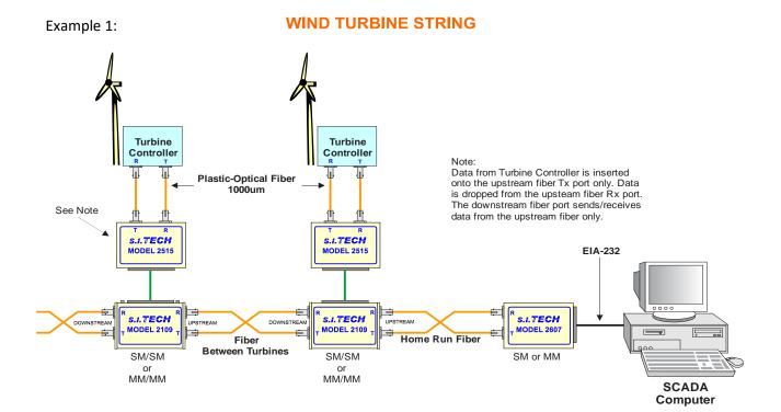
Fiber multidrop connectivity examples of wind turbine applications:
