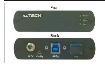
Operation Mode: USB 3.0 Input/Output Interface: USB Type B Transmission Distance: See distance chart
