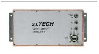
Operation Mode: USB 2.0 Input/Output Interface: USB Type B
