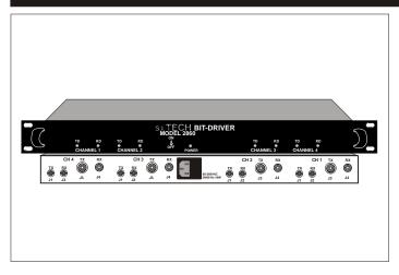
The S.I.Tech Model 2860 is designed for high speed RS-422 and TTL data communication using fiber. This system uses TRIAX and BNC connectors for interfacing to high speed network. The model 2860 provides 4 independent channels for data, clock, etc.
