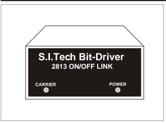
The S.I.Tech Model 2813 ON-OFF fiber optic link contains a fiber optic transmitter that generates a 10 KHz optical square wave. The 2813 fiber optic receiver detects a 10 KHz optical square wave and turns ON a relay. The relay provides 3 sets or Form C (3PDT) relay contacts available on the rear panel via screw terminals. The power input (+24 VDC or +12 VDC) is also via screw terminals.
