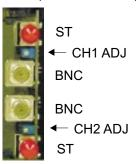
Note: Adjust (ADJ) gain in receiver CH1 and CH2 preamp for desired output (clips at 2 Vpp with 75 ohm load 4 Vpp open circuit)
