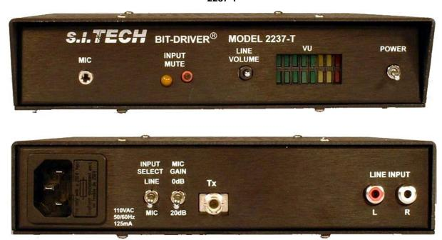
The 2237-T performs analog to digital conversion on the audio input and transmits the signal across a fiber optic cable.
