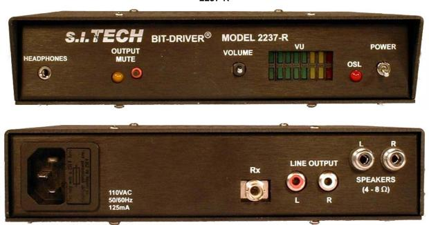
The 2237-R receives the fiber optic signal and performs digital to analog conversion for the audio output.
