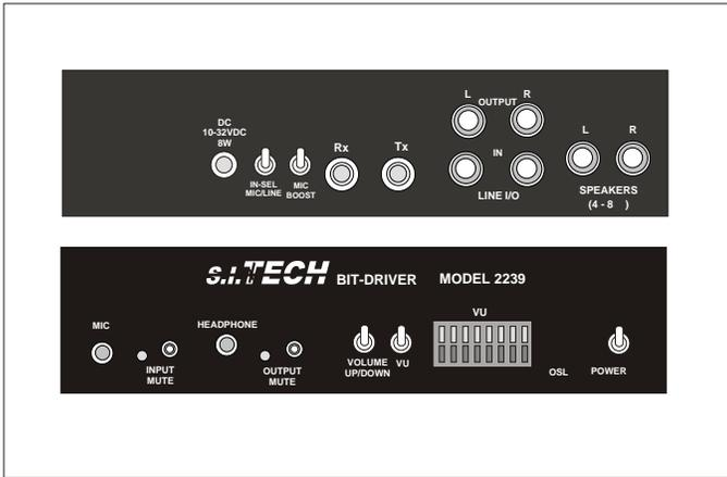
Models 2239 provides two-way stereo audio over fiber. Typical applications include paging systems, music distribution, and control with audio tones, two way audio communication.
